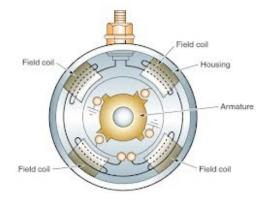
The starter in your vehicle does not uses permanent magnets, instead it uses field coils to energize and create the magnetic force and these types of motors are designed to turn in one direction only regardless of polarity. (See image)
