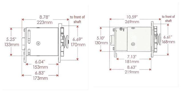
commonly found on latter model engines. To determine if you have long or short case measure the distance between the generator mounting ears.
