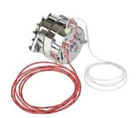
Shows 3 wire alternator connection, the white wire is the one with the diode and connects to switched 12 volts. Red wire connects directly to the battery positive side.
