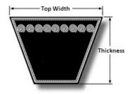
Early engines came with different width generator V belts depending on make model and year, these pulleys range from 3/8" 1/2" 5/8" 3/4", to select the correct pulley for your alternator measure the top width of the belt. All these size pulleys are available for alternators.
