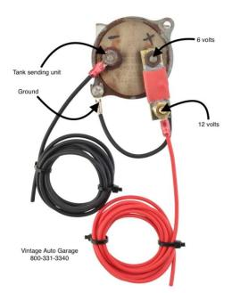
Shown above with optional wiring kit WK-VREG which includes black wire, red wire, and nylon ring terminals.
