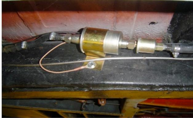
Next you will wire the power side. We have supplied 15 red wire and 10 feet of protective loom. Before you attach the wire run it thru the loom. This will protect the wire from any mishaps that will render it unusable. You will butt connect the red wire to remaining wire on the fuel pump.
