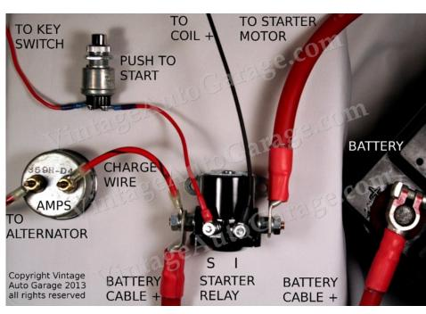
Take the other end of the long red wire and connect directly to one terminal of the ammeter, cut to size, and install small ring connector. Take the remaining length of red 10 gauge wire install ring connectors and attach one side to the opposite side of the ammeter, and the other end to the
